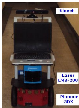
Figura 8.17: Experimento 05 - Pioneer 3DX com sensores laser (LMS-200) e kinect .
