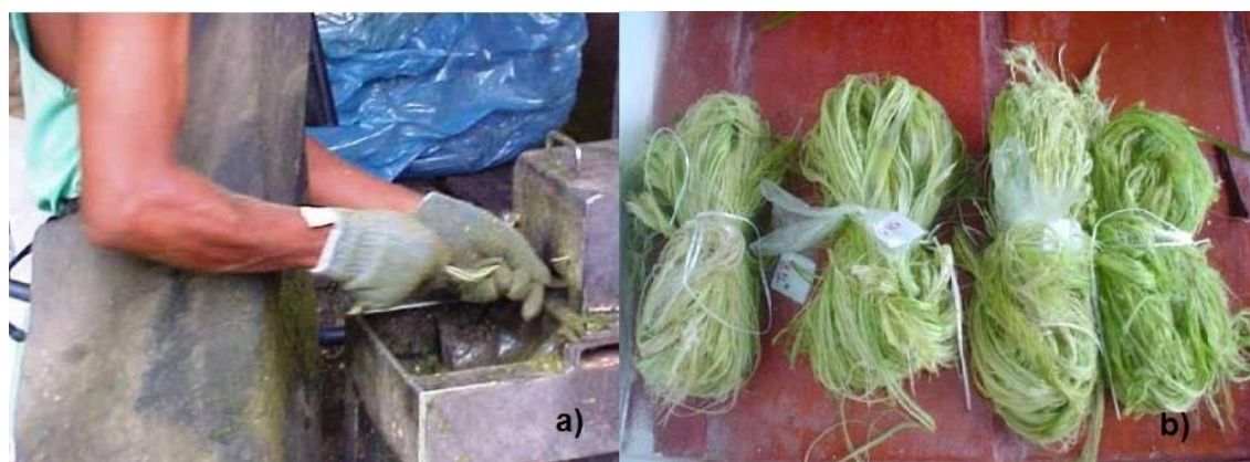
FIG. 3.8: Processo de moagem (a) e as fibras processadas (b) (John, 2016).
